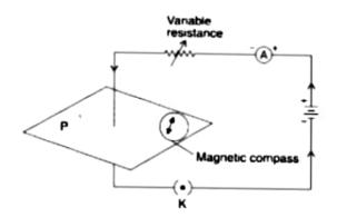
A right-hand thumb rule is applied to find the direction of these field lines. Imagine that you are holding a current-carrying straight conductor in your right hand such that the thumb points towards the direction of the current. Then your fingers will wrap around the conductor in the direction of the field lines of the magnetic field.
